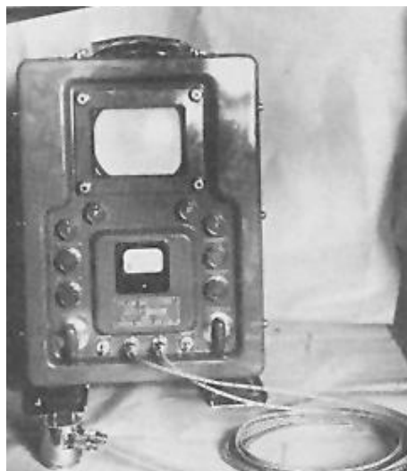
Figure 1-7 The first A-mode scanner that Uchida built in the late 1940's.
