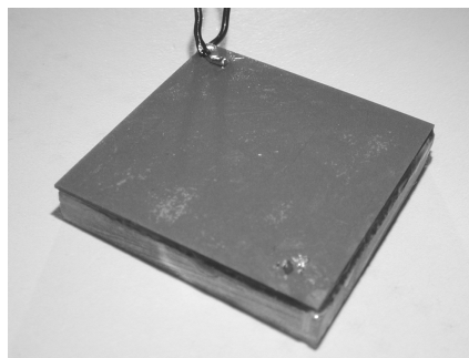
Figure 4-4 Photograph of the large single-element PXE-5 transducer with an epoxy backing.
